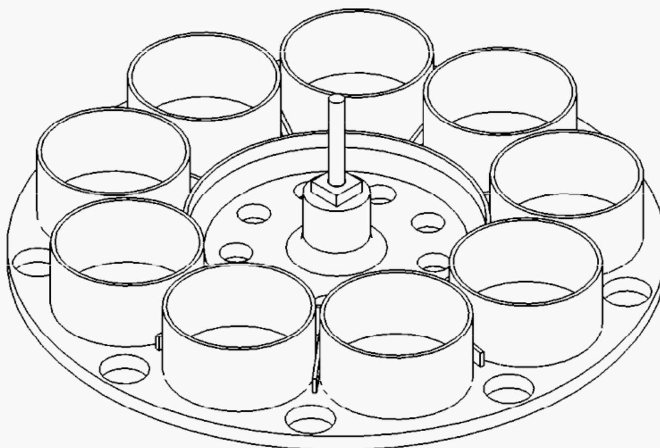
**Figure 1b — 3D representation of the aluminium shelf (example)**
