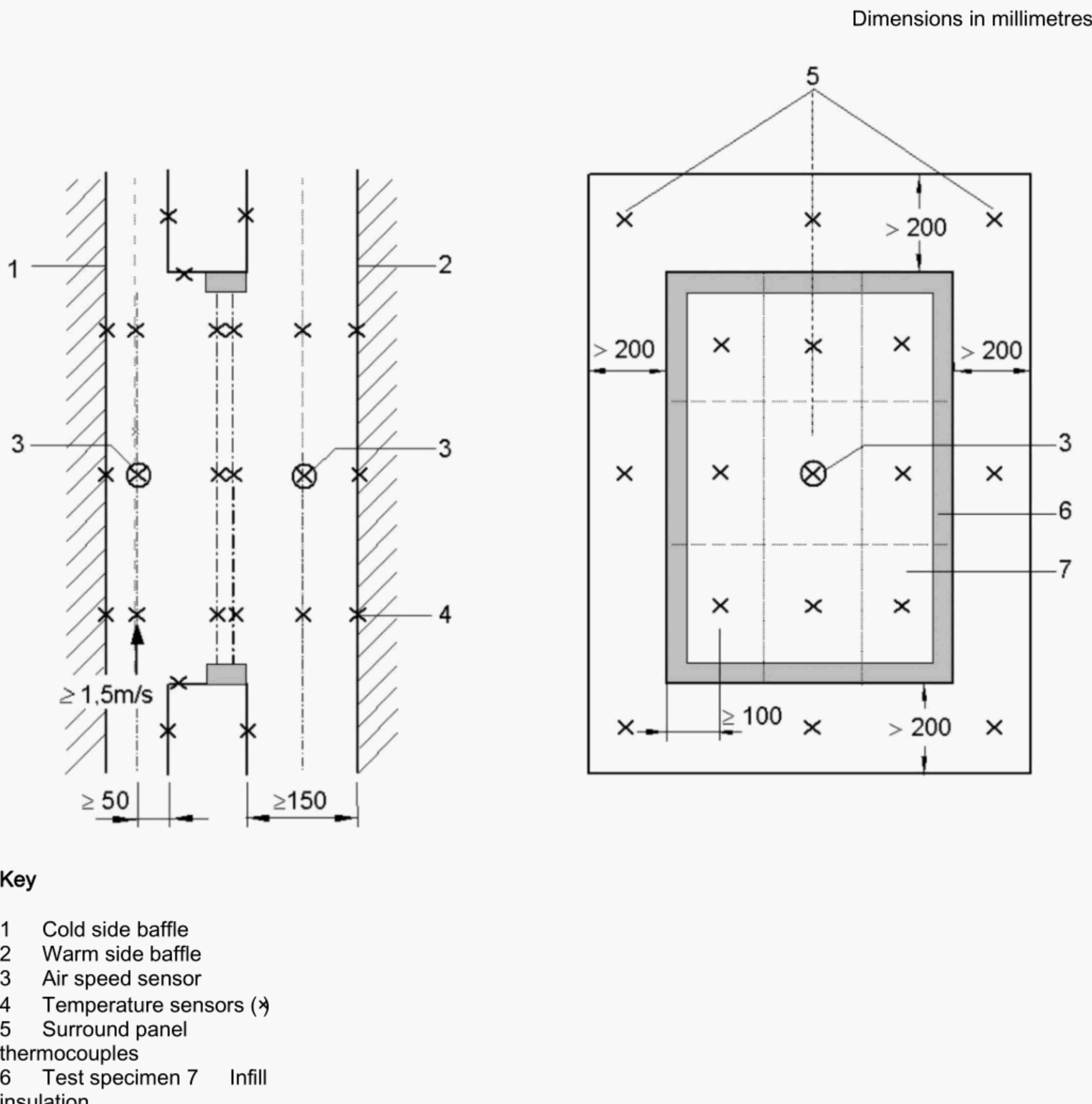
Figure 6 — Location of temperature and air speed sensors for measurements on complete frames for windows and doors
