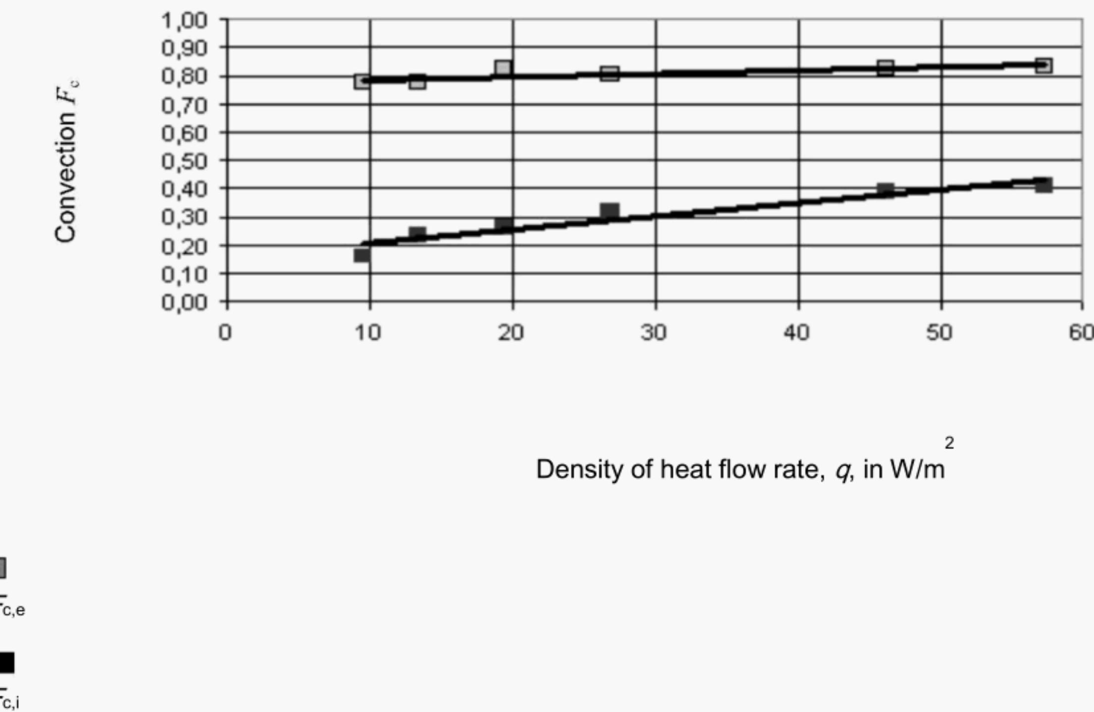
Figure C.3 — Convective fractions-cold side and warm side
