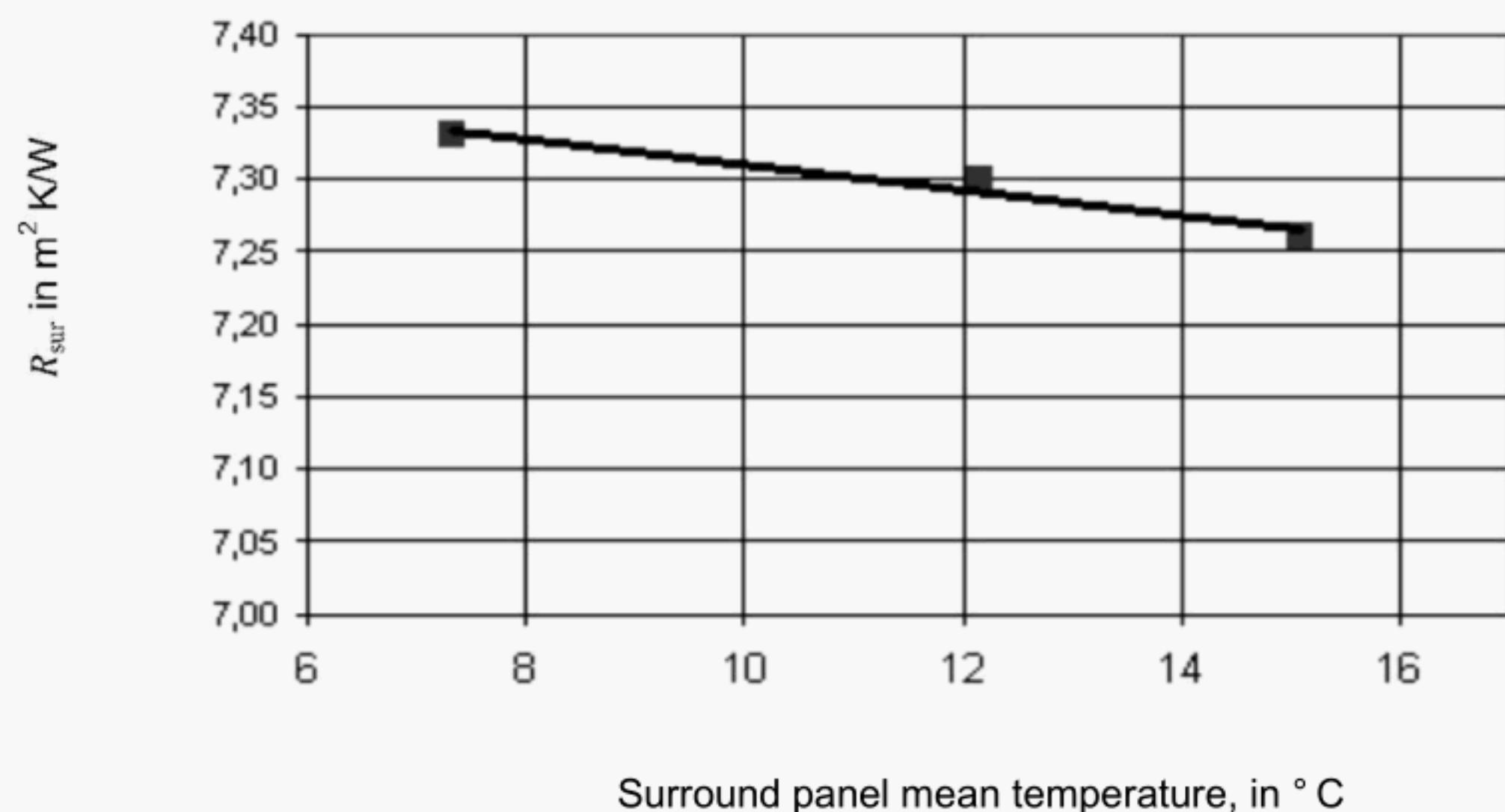
Figure C.1 — Thermal resistance of the surround panel
